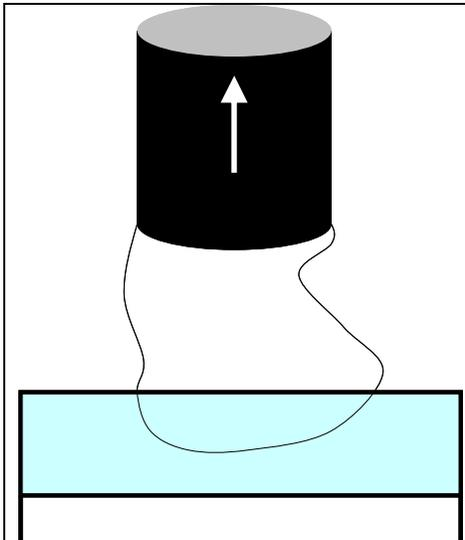
Figure 1 - Setup for soap film generation
