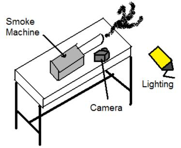
Fog from the fog machine is the only visible material used. This is a mixture of glycol and water. The fog machine heats up and the liquid is pumped through a heat exchanger which evaporates the liquid which forms a think smoke like fog. The lighting used was a small halogen free standing light. No flash on the camera was used.
