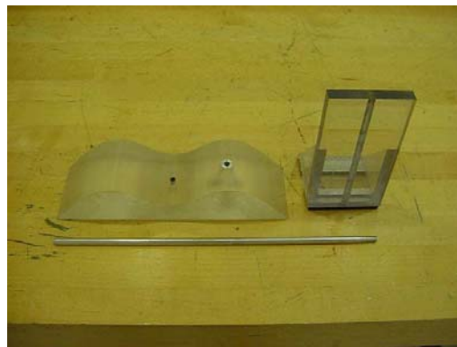
Figure 1. Left item is the double hump weir; right is the vertical wall weir. The small holes in both weirs allows for dye to be injected out into the flowing water.
