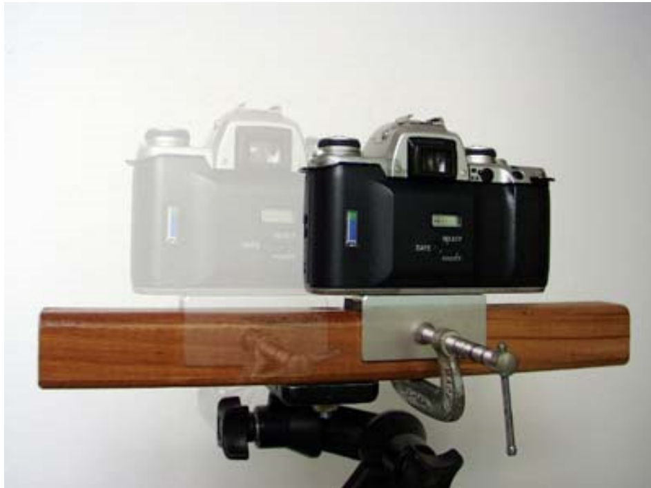
Figure 3: Stereoscopic Image setup using simple slide bar. [8]
