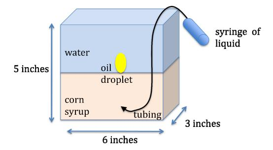
Figure 1 shows the liquid of interest being pumped into the corn syrup, water system. Approximate length scales are shown. The oil droplet's position in the image is also shown.
