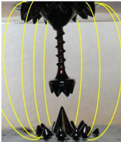
Figure 2: Magnetic Field around edges of ferrofluid on edges of magnets (not pictured)
