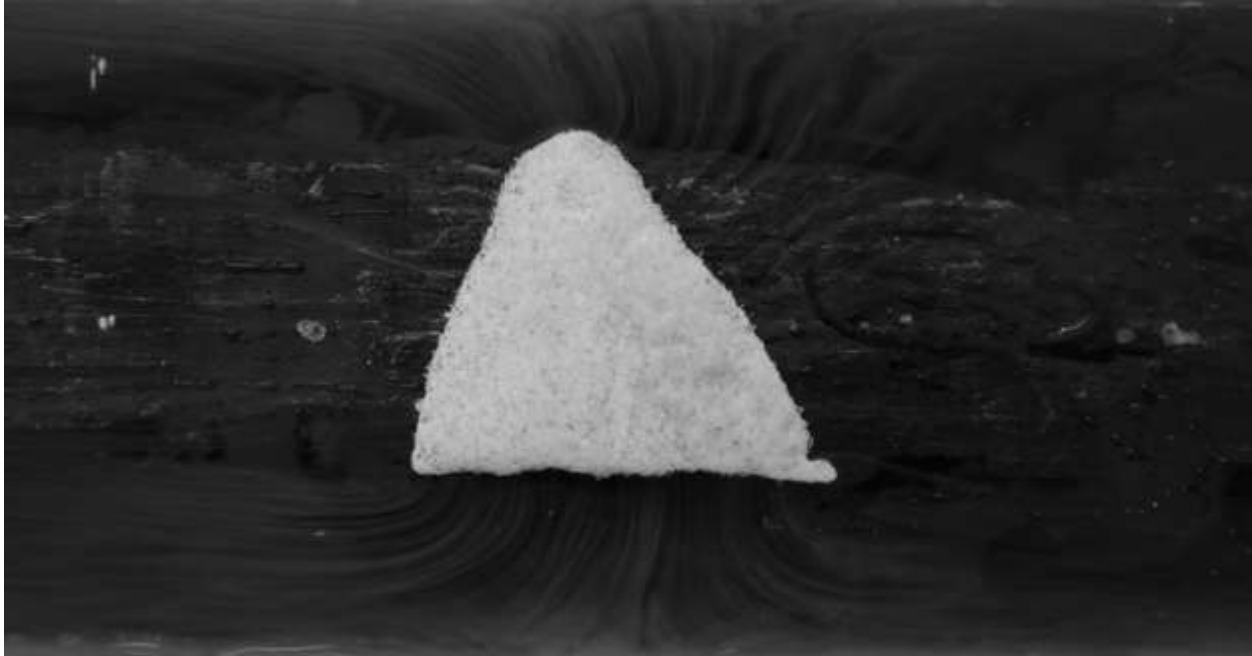
Figure 1. Dry sublimation forming laminar streamlines against a dark background.
