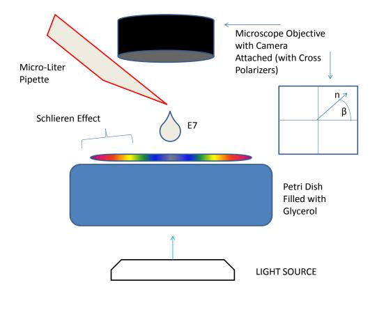
The experimental setup I used can be referenced in the following schematic below.
