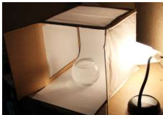
Figure 3- Light box and Fish bowl showing light source placement
