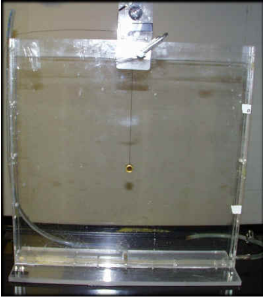
6) Capillary waves - visualization using a view graph projector.
