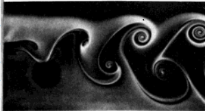
94. Kármán vortex street behind a circular cylinder at Re=1400 . Water is flowing at 1.4 \text{ cm/s} past a cylinder of diameter 1 \text{ cm} . Integrated smoke lines are shown by electrolytic precipitation of a white cobalt salt smoke, illuminated
