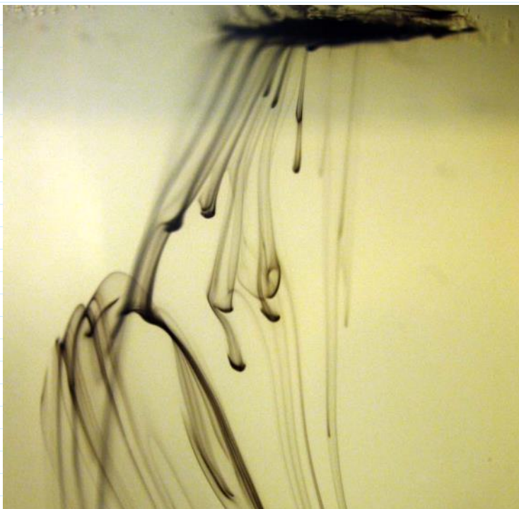
India ink falling through water shows the Rayleigh-Taylor instability. Gordon Browning. Get Wet Fall 07.
