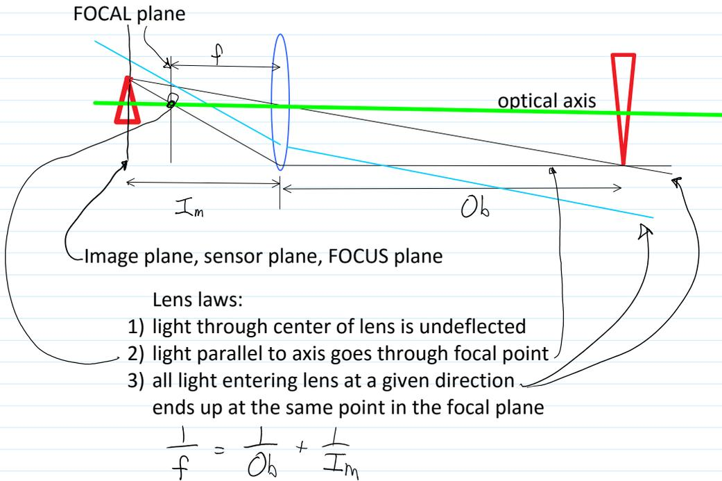
As object moves closer, lens must move away from sensor plane to maintain focus. Mechanical limit defines near focus distance.
