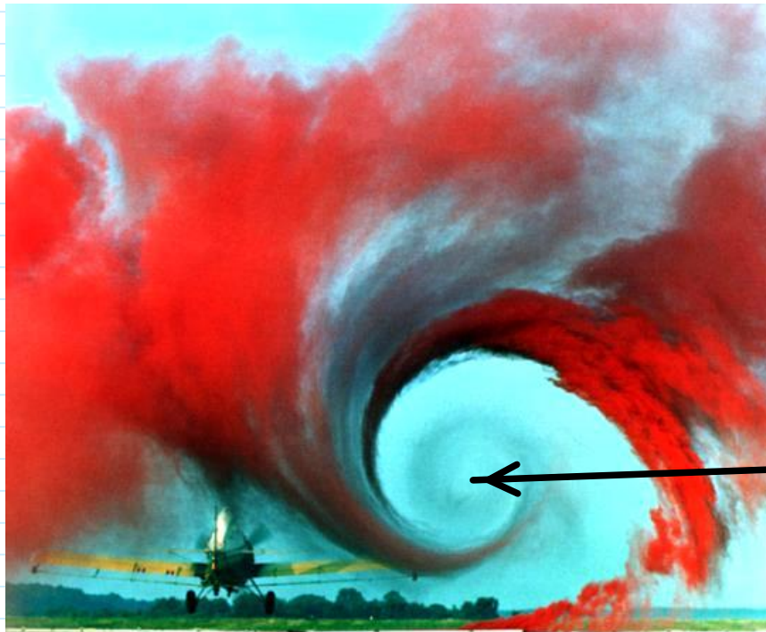
Wake Vortex Study at Wallops Island NASA Langley Research Center 5/4/1990 Image # EL-1996-00130 "NASA wing tip vortex. Information for ID # EL-1996-00130," n.d., http://lisar.larc.nasa.gov/UTILS/info.cgi?id=EL-1996-00130 .
