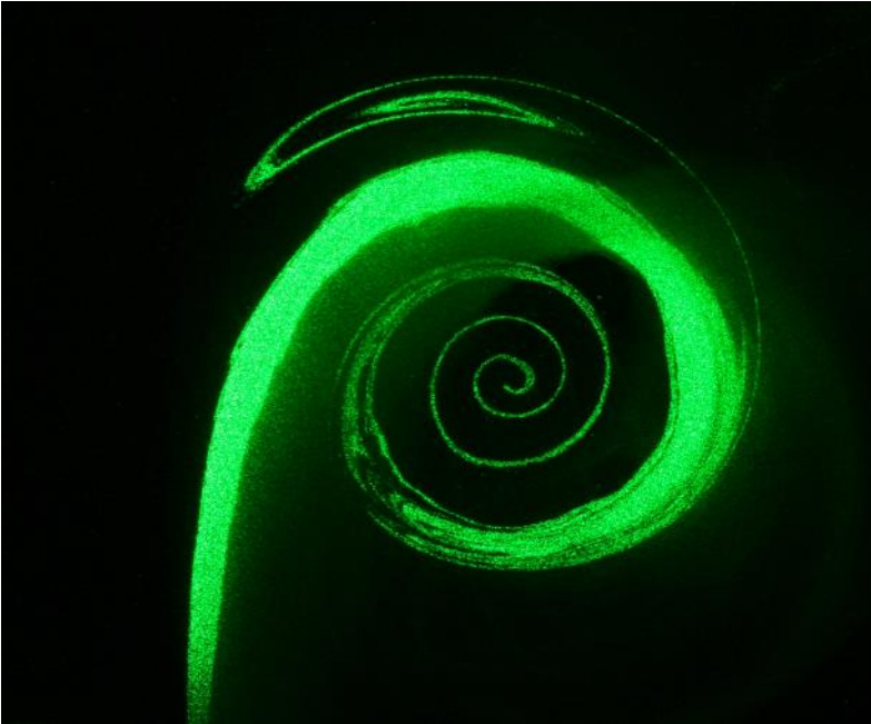
Stage fog illuminated by a sheet of laser light forms a suddenly started laminar planar jet at Re = 330 . Tanner Ladtchow, Geneva Wilkesanders, Tim Read, Andrea Fabri. Team Project 3, 2006
