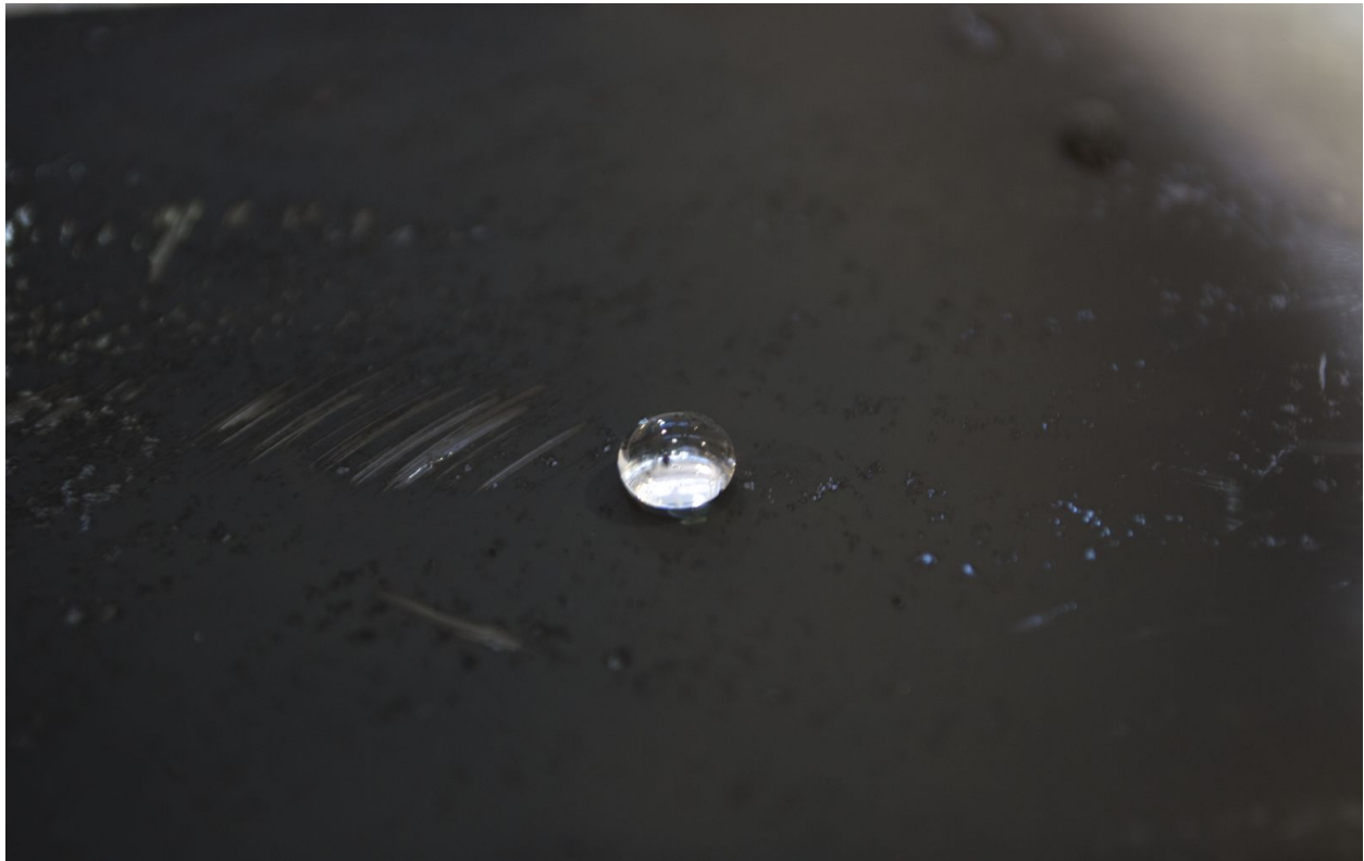
Figure 1. Single drop on a superhydrophobic surface
