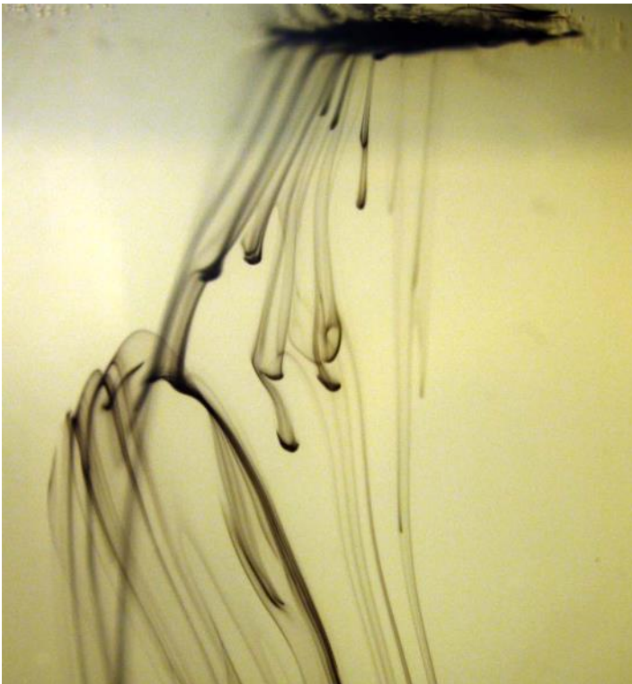
India ink falling through water shows the Rayleigh-Taylor instability. Gordon Browning. Get Wet Fall 07.
