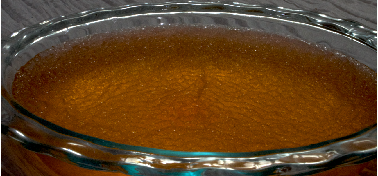
Figure 1: Gelatin wrinkles on the surface of colored water. Photographed by Riley Menke, assisted by Maddie Leaver
