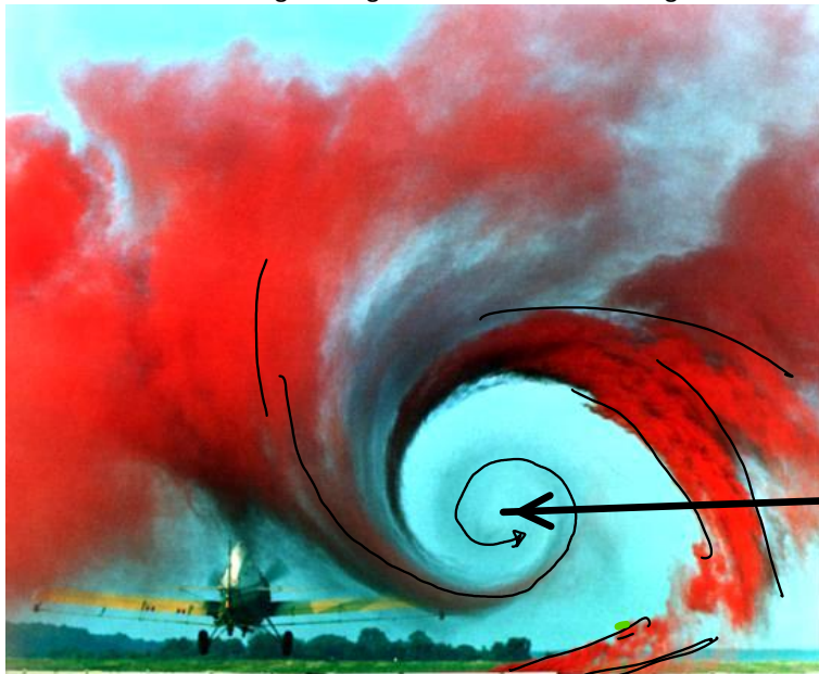
NASA Wake Vortex Study at Wallops Island NASA Langley Research Center 5/4/1990 Image # EL-1996-00130 "NASA wing tip vortex. Information for ID # EL-1996-00130," n.d., http://lisar.larc.nasa.gov/UTILS/info.cgi?id=EL-1996-00130 .
