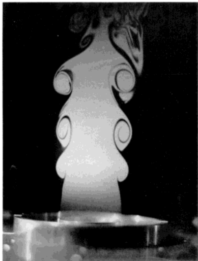
FIGURE 4 Example of tomography. Free jet, 1.2 m/s, issuing into stagnant room air.
