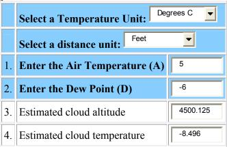
This calculation is based on the assumption that there is a linear relationship between cloud height and cloud temp. The linear relations used are listed below:
