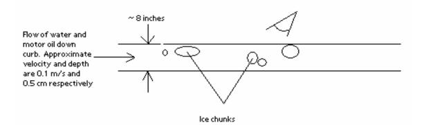
The field of view in this experiment is small, being only about 2" wide by 3" long. The flow rate of the water is estimated to be 0.1 meters per second, and the depth of the water/oil is about half a centimeter. With the consideration of the velocity of the fluid and the shutter speed of the camera, the fluid would have moved a distance of 0.625 millimeters. When compared to the field of view, this movement is very small, and so
