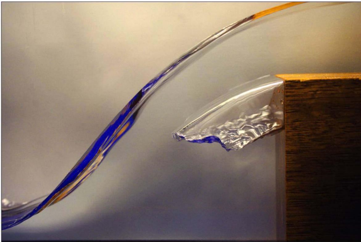
Figure 1: Photo of bubble trapped beneath water flowing over broad crested weir.
