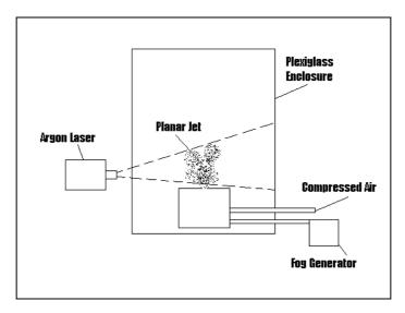
For the given setup we can estimate Reynolds numbers using the following equation:
