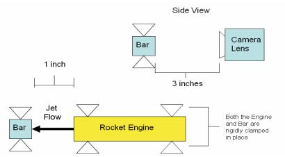
The apparatus used to capture this flow.
