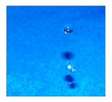
At the nozzle, water is pulled down by gravity and forms a neck. When the neck "snaps", the water tension pulls the water into a spherical shape. This shape is distorted as it falls through air, but since the drop distance was relatively short, the drop distortion was negligible. While this setup yielded more constant results, they were not as repeatable as I would have liked. In order to solve this I added an astable 555 timer circuit to open and close the valve.
