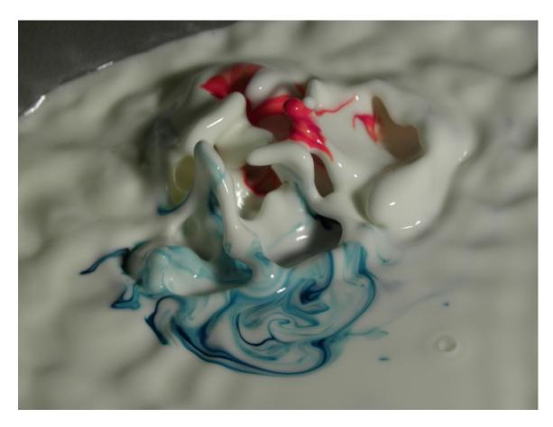
Working with the vibrating table, properties of non-Newtonian fluid can be observed for MCEN 4228 Flow Visualization, Group Assignment #2. Non-Newtonian fluid was created using corn starch and water and placed on a vibrating table. The table was vibrated at a certain frequency and the fluid acted in a fascinating way. A camera was used to take still images of the interesting flow that was created when the non-Newtonian fluid was place on the vibrating table.
