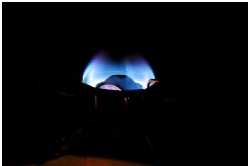
Figure 1. Pressurized stove burning white-gas and generating a blue-violet oxygen rich flame
