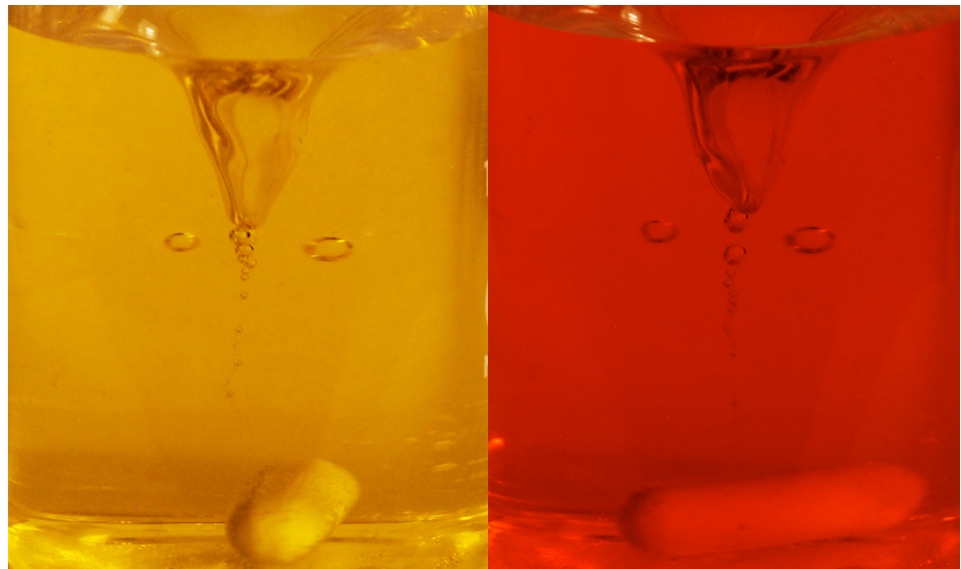
Figure 15: The two images directly before and after the final photograph reveal satellite bubbles trapped by an unknown force. These bubbles are also in the final photograph.
