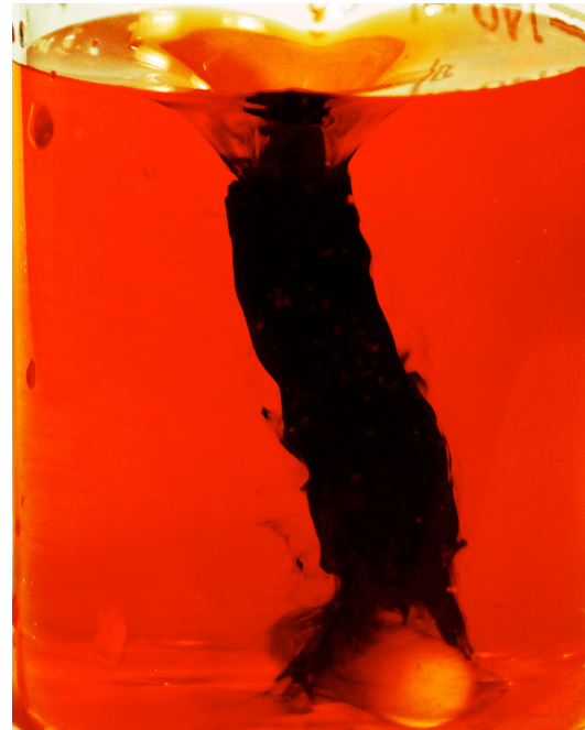
Figure 7: Blue dye remains in the jet with minimal mixing into the red dye
