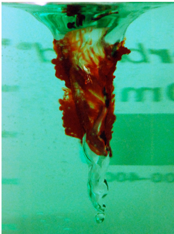
Figure 10: Red dye stays close to the cone as it gets pulled down and around
