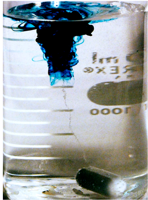
Figure 9: Buoyant bubbles fight against anticentrifugal forces and the downward pulling jet
