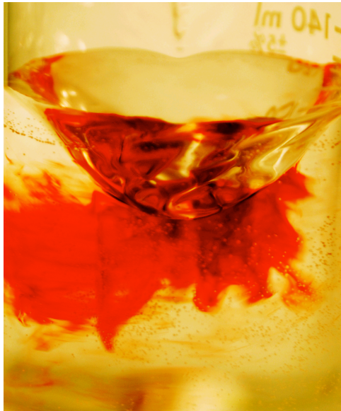
Figure 6: Wider vortex created by using a larger magnetic stirrer
