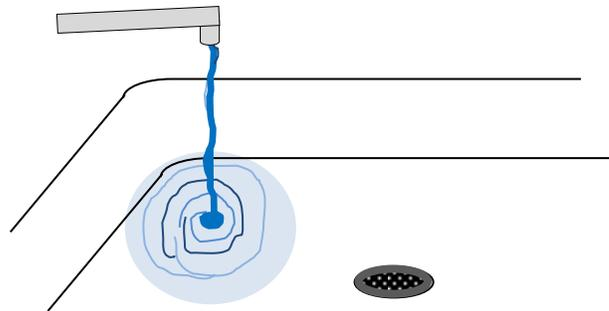
Varying the pressure of the faucet I was able to obtain different properties in the stream of the flow. In particular I wanted to capture the water splashing as it hit the basin of my sink. The flow was low enough where the water did not appear to be forced out of the faucet but was flowing freely. A flow with a low Reynolds number is considered to be steady and non-turbulent or a laminar flow. The Reynolds number is calculated to be:
