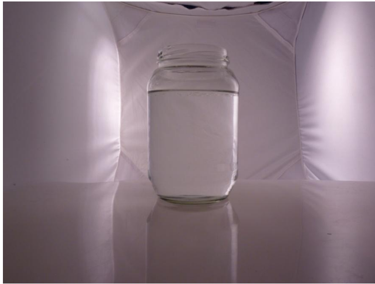
Figure 4: Jar setup inside white photography box with lighting on both sides
