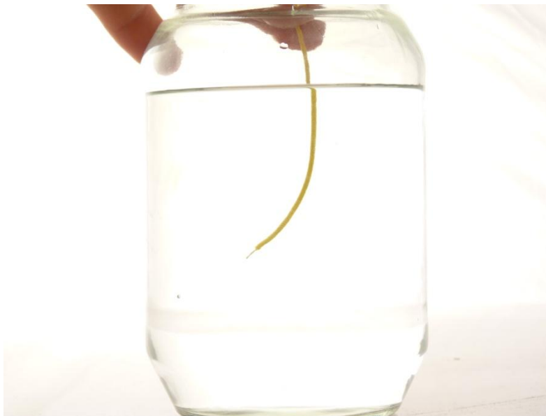
Figure 5: Straight jumper wire used for manual focusing. Taken at long exposure.
