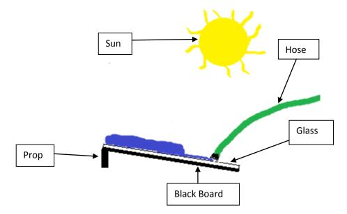
By varying the height of the prop and the distance of the hose from the surface of the glass, the point at which the hydraulic flux occurs could be varied. The camera angle used was about 20 degrees above the surface of the glass and of the same perspective shown above.
