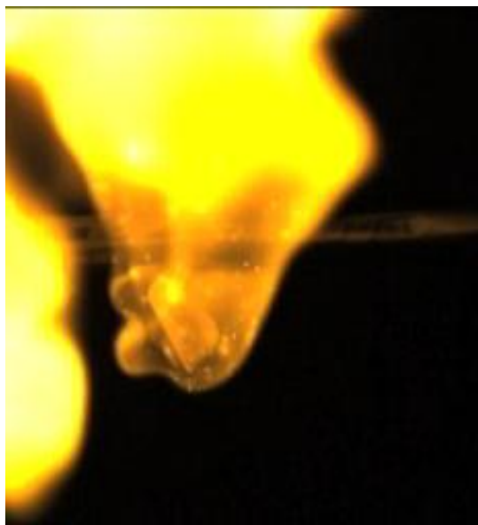
Figure 3: Pyrolysis of nitrocellulose while falling
