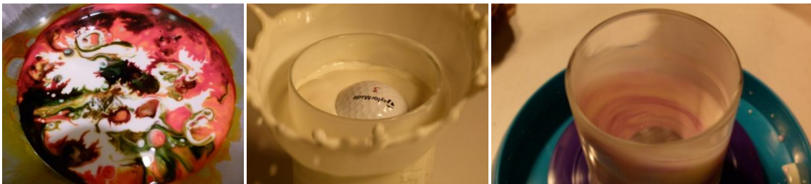
Figure 1. Experimental photos of oobleck with folded-in food dye (left), a golf ball tossed into thinned oobleck (center) and dyed fluid rotating in a Spin Art toy (right).
