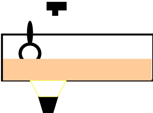
The figure displays the set up. The light is below emitting light through the tank and the mixture. The camera is pointing down at the mixture directly pointing towards the light. A mirror was placed into the mixture and a paddle motion was created
