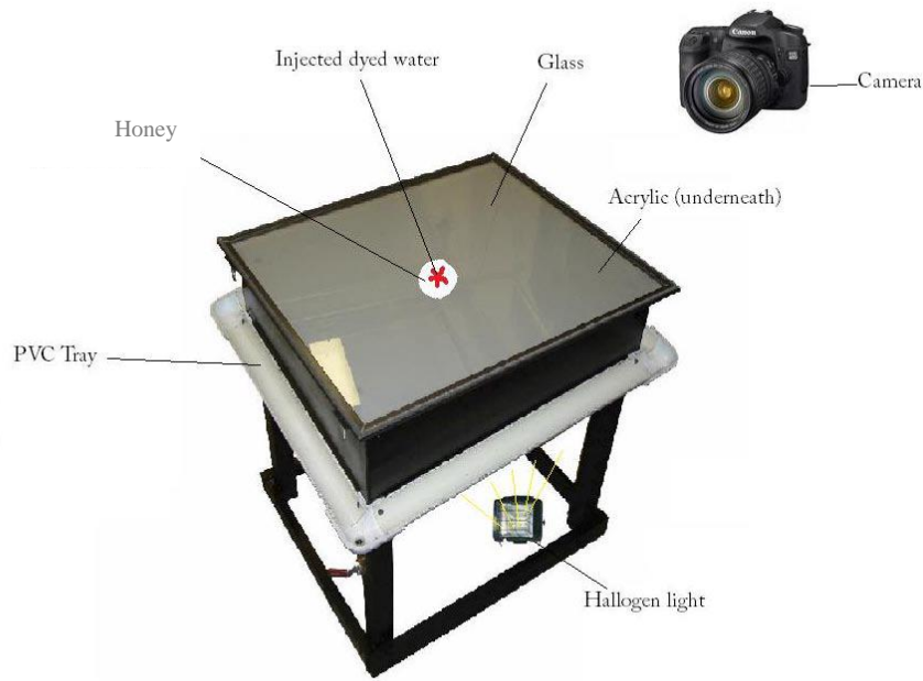
Figure 1: Hele-Shaw cell used in the setup of this image
