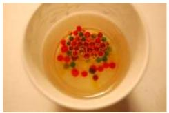
*Figure 3 left* shows the "Pre-Photoshop" image. The bubbles are small, but clear. The field of the view is about 7 cm. The distance from object to lens was about 10 cm. The image was captured with a Nikon D40 DSLR Camera. The camera settings were ISO 1300, F 5.6, and 1/50 shutter speed (3008 x 2000 pixels).
