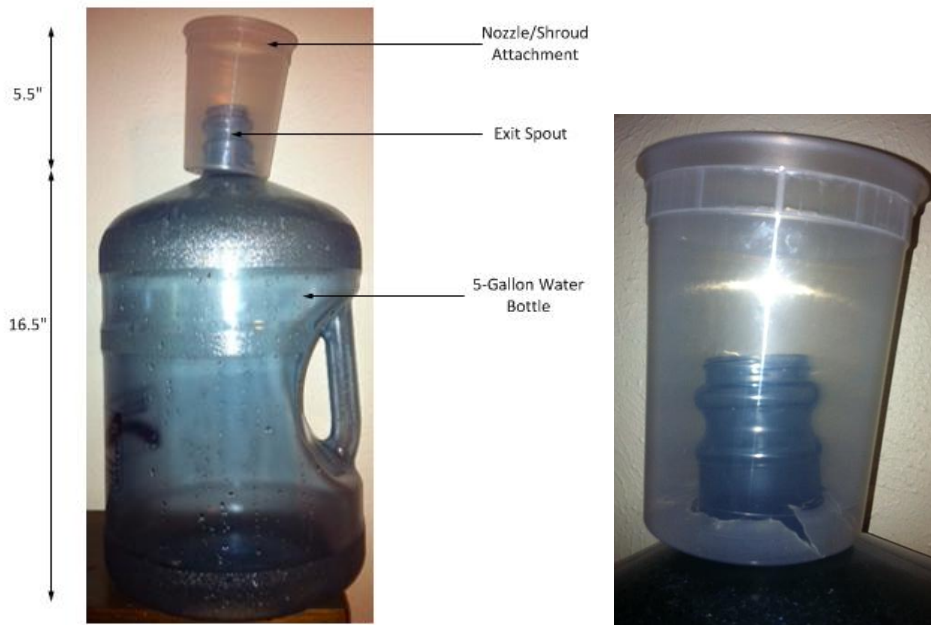
Figure 1: (Left) Entire Experimental Set-up, (Right) Close-up Detail of Nozzle/Shroud Attachment
