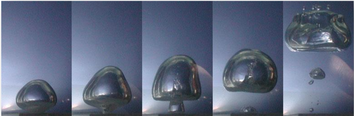
Figure 4 Creation of bubble sequence 5
