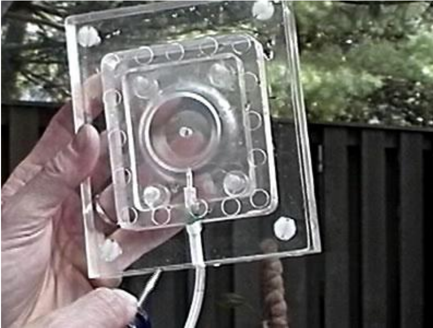
Figure A. Bubble ring generator 6
