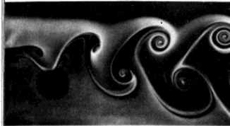
94. Kármán vortex street behind a circular cylinder at Re=140 . Water is flowing at 1.4 cm/s past a cylinder of diameter 1 cm. Integrated streaklines are shown by electrolytic precipitation of a white colloidal smoke, illuminated
