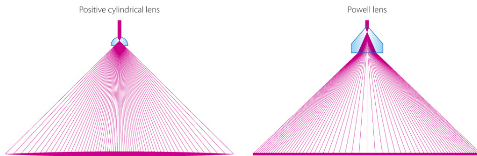
Figure 14: Cylindrical lens vs Powell lens [15]
