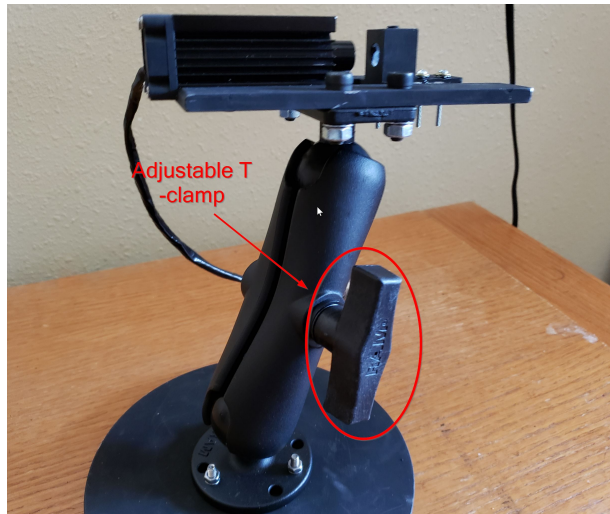
Figure 15: T-clamp for adjusting the fixture
