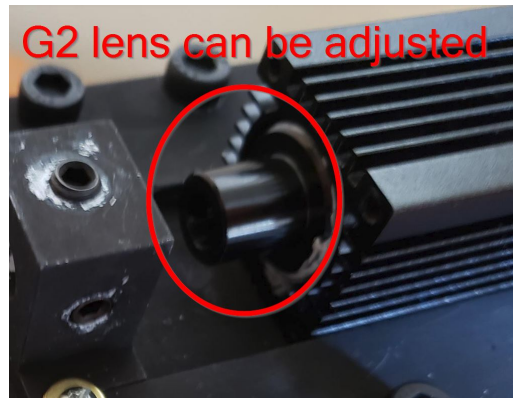
Figure 17: The G2 lens can be adjusted by turning the barrel
