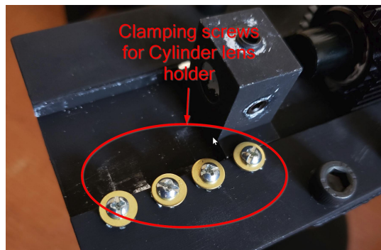
Figure 16: Screws for holding the lens holder down
