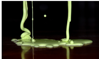
Oobleck: Pouring a cornstarch/water mixture shows non-Newtonian behavior, as the faster moving fluid is 'stiffer' than the slower, pooled mixture. Robert Irmiger
