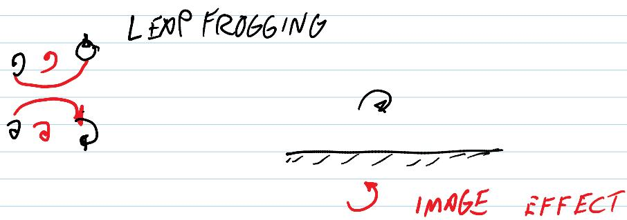
Contrails are long parallel vortexes. Loop forms starting with takeoff, ends on landing
