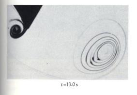
**80. Starting vortex on a wedge.** A piston drives water with almost constant speed normal to the axis of a wedge of 30° semi-vertex angle. Neutrally buoyant dye is injected into the water from small holes in the wedge surface. The characteristic Reynolds number is of order 1000. The piston stops at 12.5 s, producing a stopping vortex in the last photograph. *Pullin & Perry* 1980
