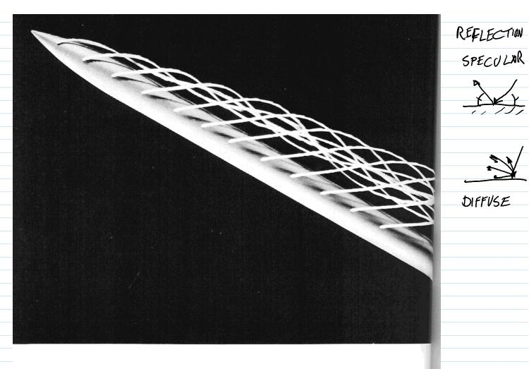
87. Attached vortex pair behind an inclined slender body. A long ogive-cylinder is inclined at 30° to water flowing at 4 cm/s. At this angle of attack a symmetric pair of vortices forms on the lee side of the body. Colored fluid emitted under slight pressure from 0.3-mm holes spirals around the core of the nearer vortex. The Reynolds number is 400 based on the diameter of 1 cm. *Fiechter 1969*
