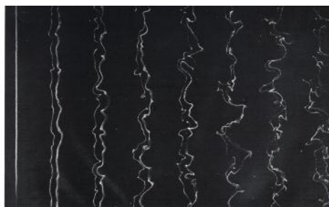
154. Growth of material lines in isotropic turbulence. A fine platinum wire at the left is stretched across a water tunnel 35 mesh lengths behind a turbulence-generating grid. The Reynolds number is 1300 based on grid rod diam-
