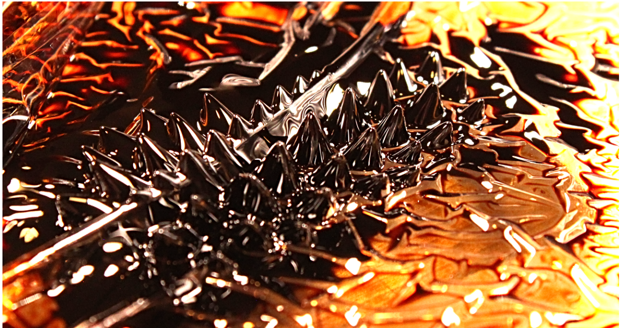
Figure 1, Depiction of the Flow Phenomenon of Ferrofluid in a clear dish under the effect of a magnetic field
