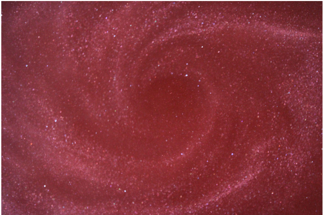
Figure 4. Original Image of Vortex Formed by Stirring Shimmering Water in a Container
