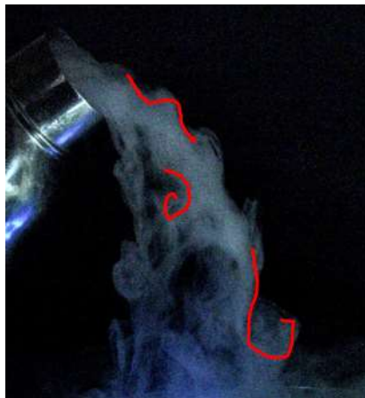
Figure 2. Highlights the Kelvin-Helmholtz Instability pattern in the fluid flow of CO 2 gas.
