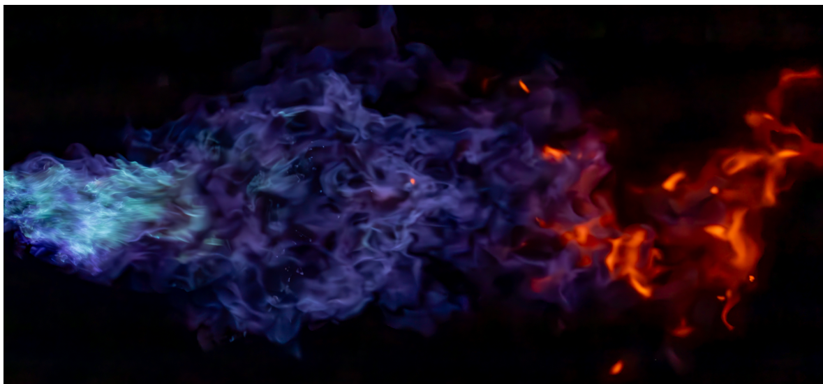
Figure 3.1.3: Full flow premixed propane flame, does not impact water
